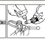
STEP 4 Dip the nipple end into a lubricant. Refer to step 2. (Light weight oil S.A.E. 10 or 20)
