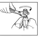
**STEP 5** Turn the stem clockwise into the hose and socket until the stem hex shoulders. against the ferrule.
